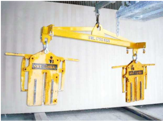
Lifting jaws set up on spreader bar
