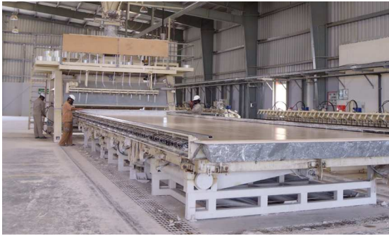
Rapidwall panel manufacture
