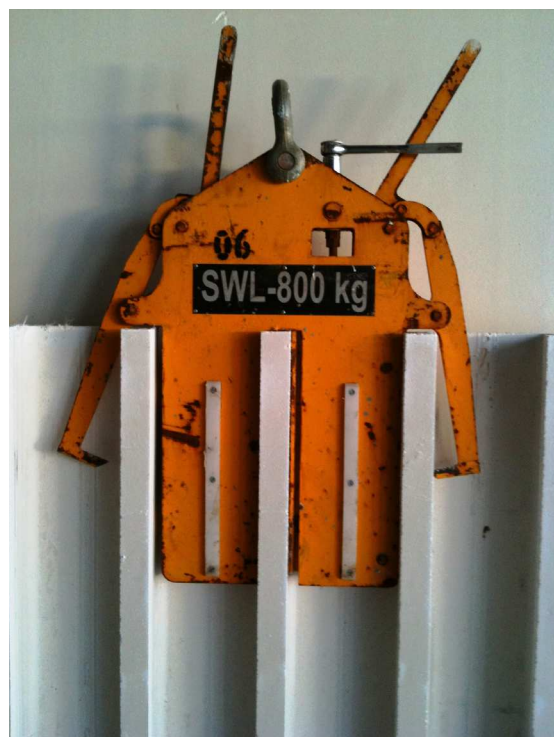
Lifting jaw showing clamping method
