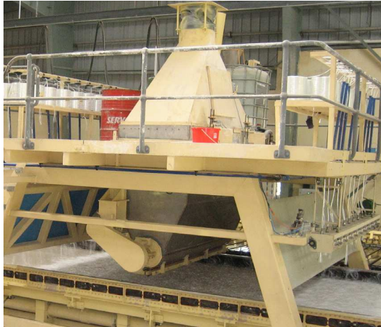
Laying fibreglass during manufacture
